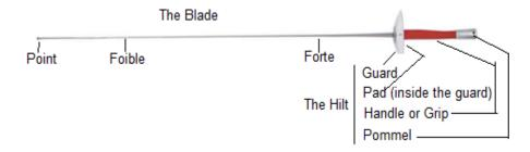
The tang is the part of the blade inside the handle and everything is held together by the pommel screwed onto the end of the tang.
